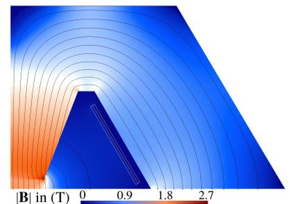
**Figure 2:** Magnetic flux density (not considering a beam pipe).
