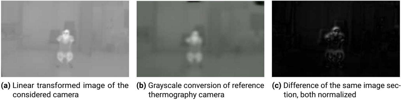
**Figure 4.5:** Comparison of known good temperature scale to presumed linear transformation
