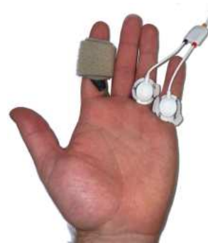
(f) Placement of cuff and electrodes on the hand.
