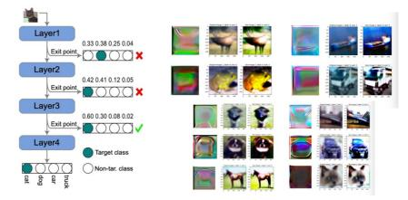
Left figure: The concept of early-exit in CNNs. Right figure: Modification of image data to enable earlier-exit in CNNs
