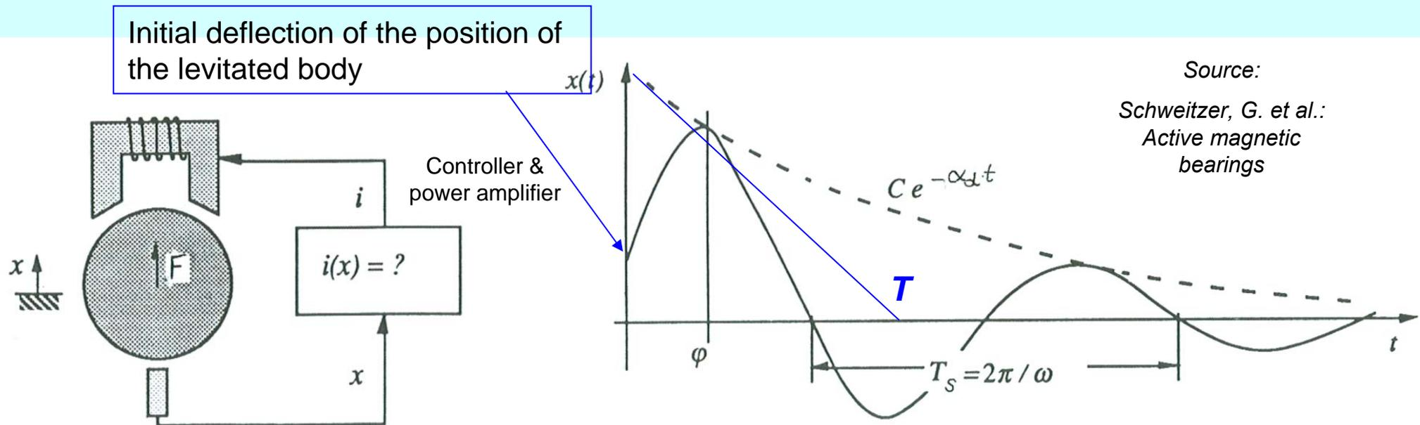
$$\frac{\alpha_d}{\omega} = 1/\sqrt{3} \Rightarrow \frac{T_s}{T} = \frac{\alpha_d}{f} = \frac{\alpha_d}{\omega} \cdot 2\pi = \frac{2\pi}{\sqrt{3}} = 3.6$$
