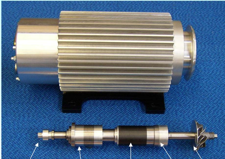
Axial sensor measuring track    Magnetic axial & radial bearing    PM-Rotor    Measuring track    Compressor runner
