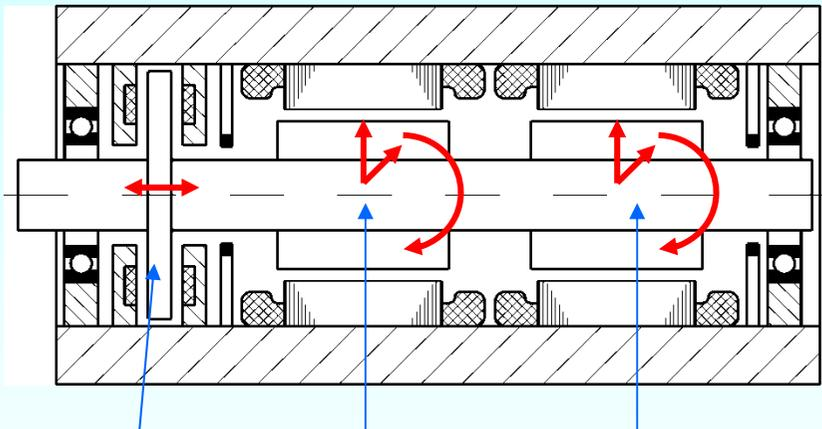
Axial bearing    Radial bearing 1    Radial bearing 2
