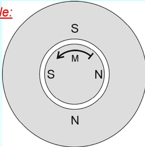
Combination of a rotor field with  $p_1$  pole pairs with a stator field of  $p_1$  pole pairs generates the torque  $M$
