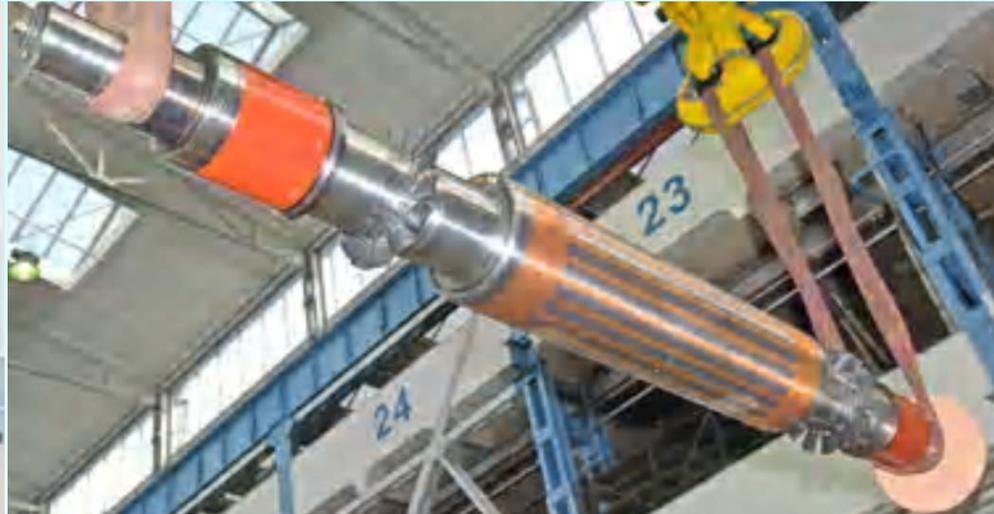
15000/min, 4 MW squirrel cage – induction motor
