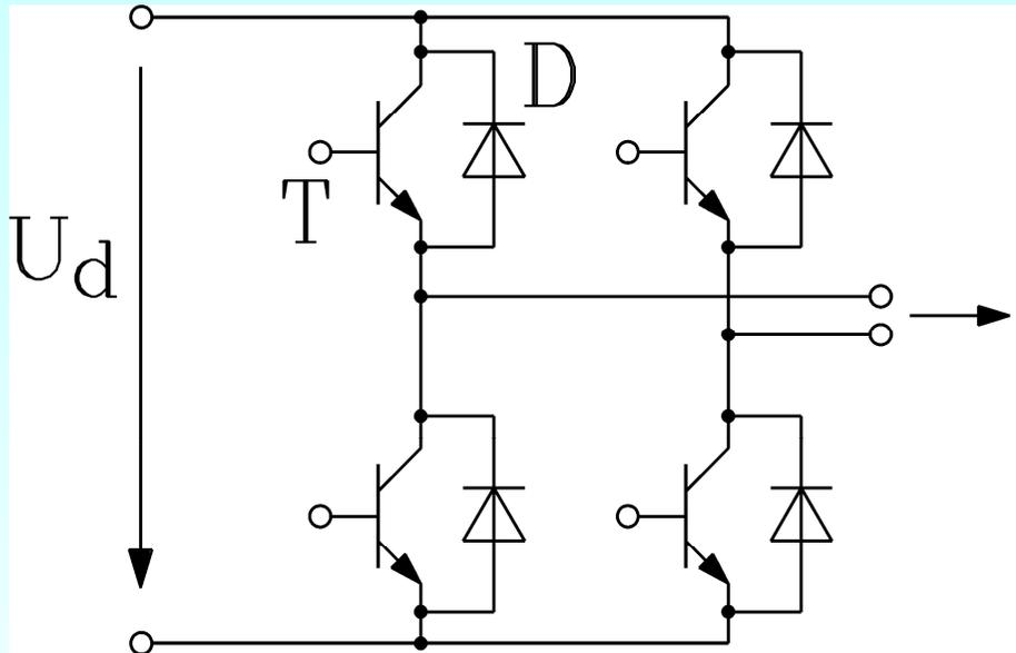
Feeding the R-L-coil system of the AMB
