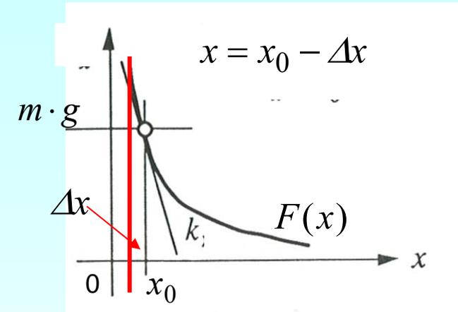
*Position deviation increases exponentially with time; the rotor does not return back to its starting operation point. The working point is unstable.*
