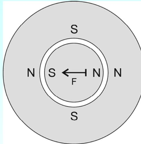
Combination of a rotor field with  $p_1$  pole pairs with a stator field with  $p_2 = p_1 \pm 1$  generates a lateral force  $F$
