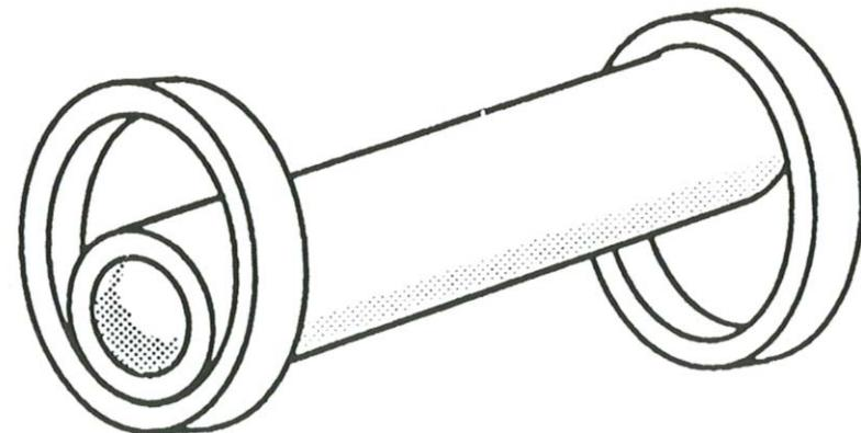
**Differential-mode** movement in the aux. bearings
