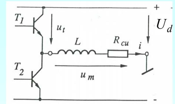
**Example:**  $\pm U_d = \pm 150 \text{ V}$ , Coil resistance  $R_{Cu} = 2 \Omega$ , max. coil current  $i = 6 \text{ A}$ :
