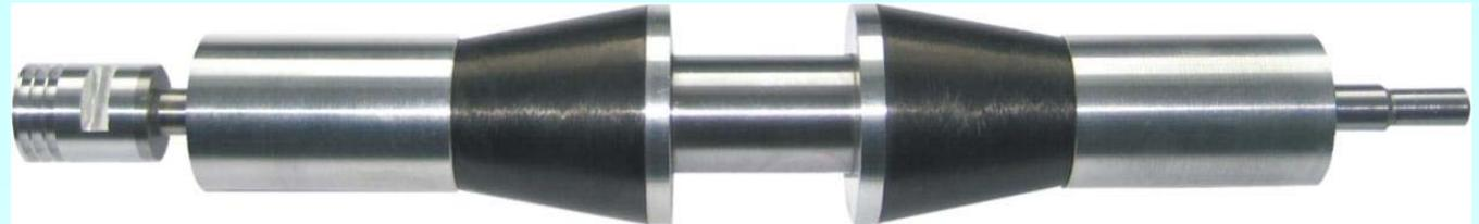
*Prototype:* 18000/min, 1 kW: Per half machine: 500 W with 2-pole drive and 4-pole levitation winding. Successfully tested!
