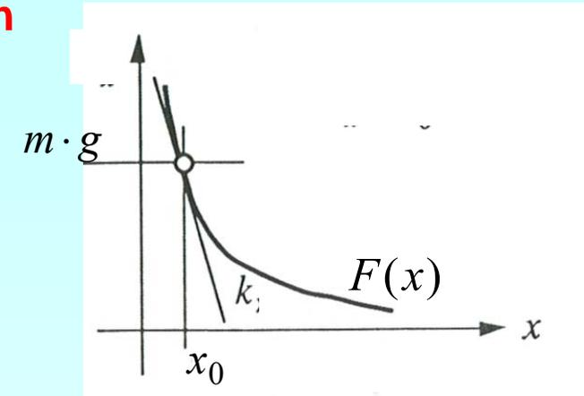
$$\left. \frac{dF}{dx} \right|_{x_0} = -\frac{F_M}{\left(1 + \left(\frac{x_0}{\Delta}\right)^2\right)^2} \cdot \frac{2x_0}{\Delta^2} = -\frac{(m \cdot g)^2}{F_M} \cdot \frac{2}{\Delta} \cdot \sqrt{\frac{F_M}{m \cdot g} - 1} = -k < 0$$
