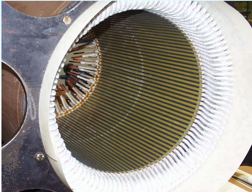
Stator winding „white = green“ before resin impregnation, q = 1.5
