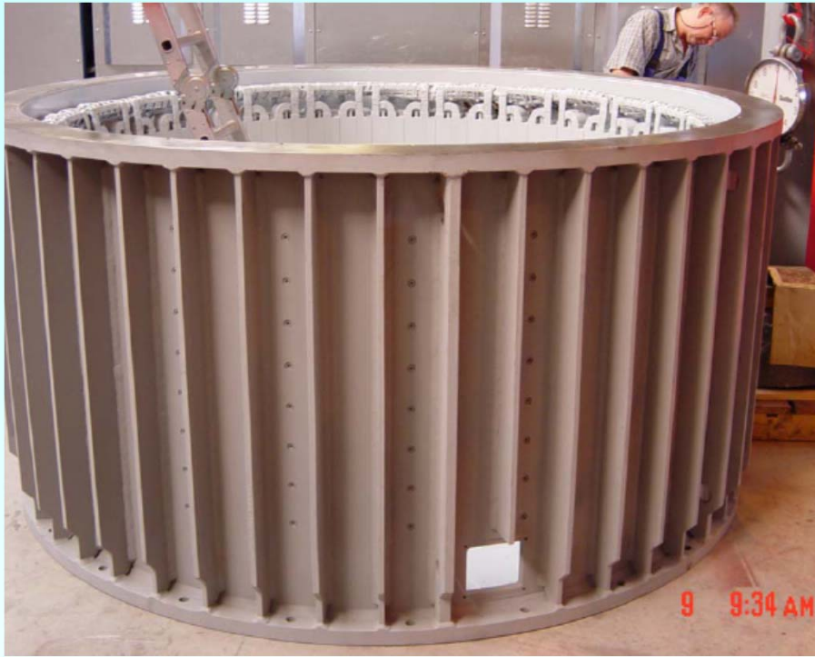
Stator manufacturing with tooth coils
