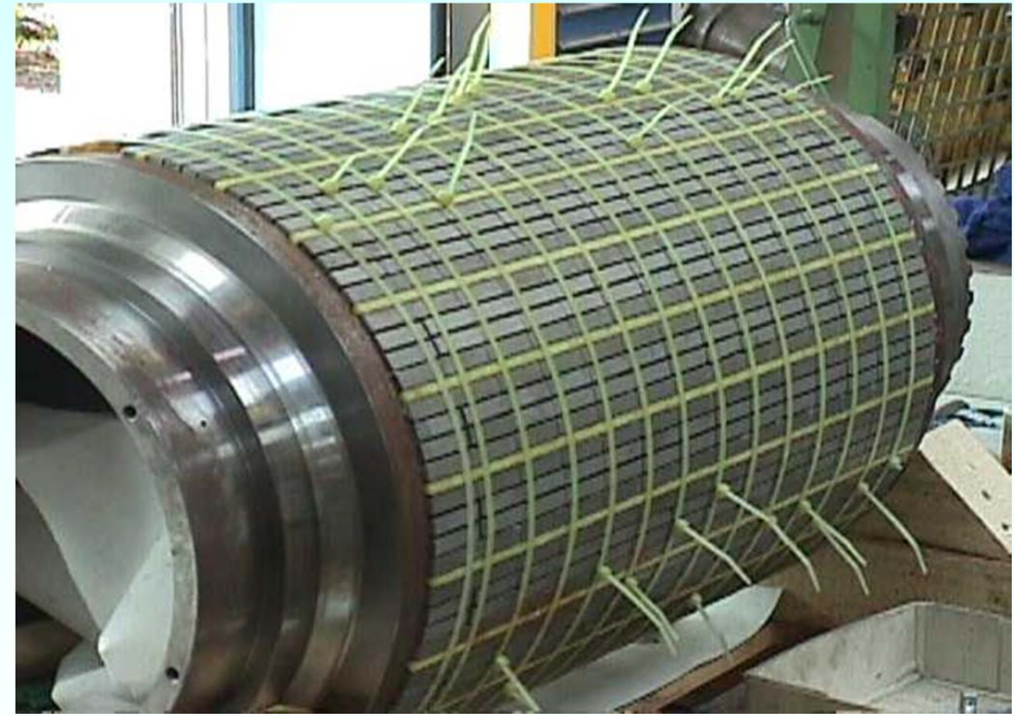
Magnets glued to rotor before bandage is wound on rotor
