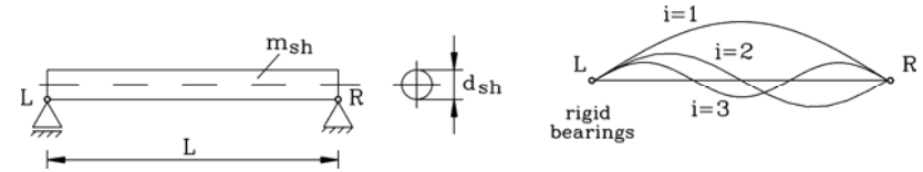
Fig. 7.1.5-3: Model of shaft as cylindrical beam, showing a spectrum of bending natural frequencies, which depend on the influence of bearing stiffness
