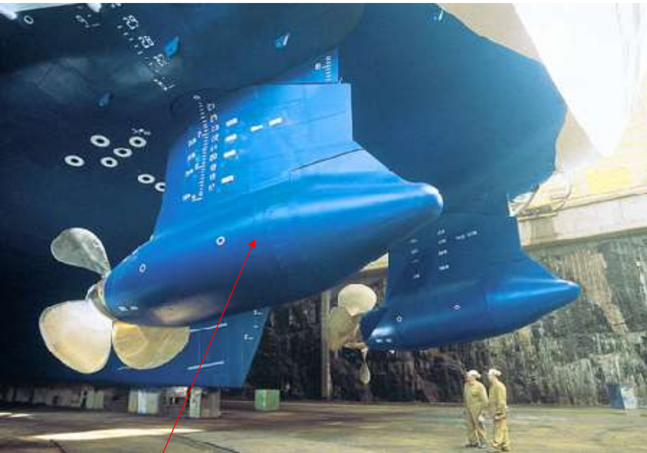
Synchronous motors inside
