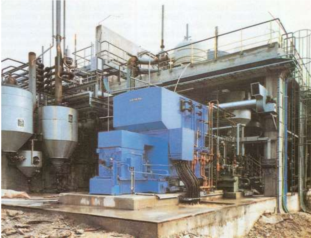
Extrusion drive 2 MW at 120 ... 1500/min at protection IP54 and explosion proof EEx e
