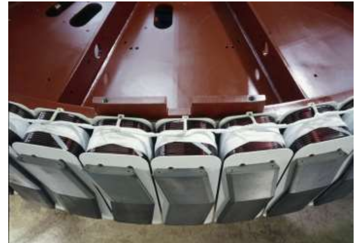
Rotor: Electrical excitation , rotor pole shoes skewed to reduce cogging. Double-skew avoids axial force
