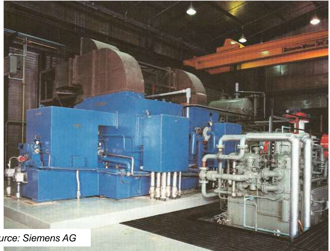
Natural gas pipeline: Gas compressor 18 MW at 5200/min, explosion proof „pressurized“ EEx p
