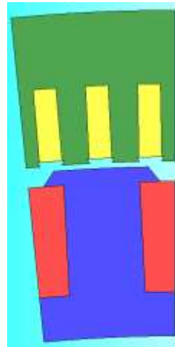
Integer-slot q = 1 stator winding, rotor electrical excitation
