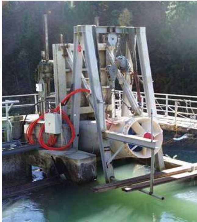
The test rig of a StrafloMatriX™ unit at the Agonitz plant, Austria
