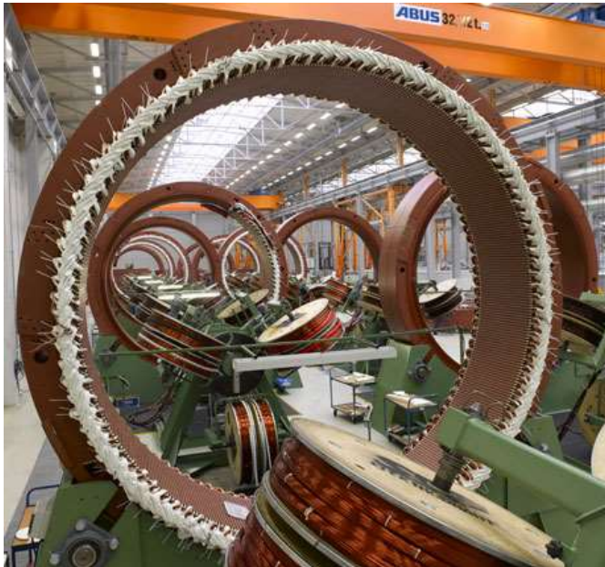
Integer-slot q = 1 round wire low voltage single layer stator 3-phase winding manufacturing
