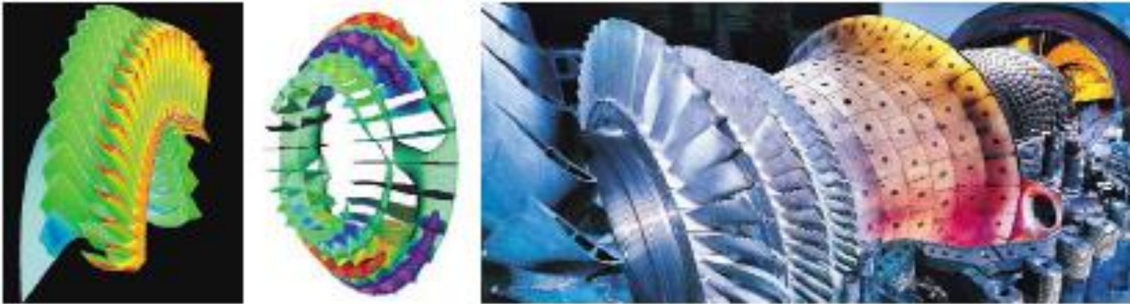
Numerical hot gas flow simulation for optimization of blade profiles in a gas turbine
