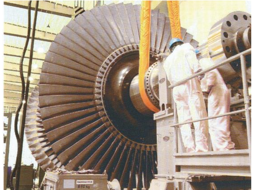
Low pressure steam turbine rotor with two-sided steam flow, made of rotor discs, total weight 260 tons
