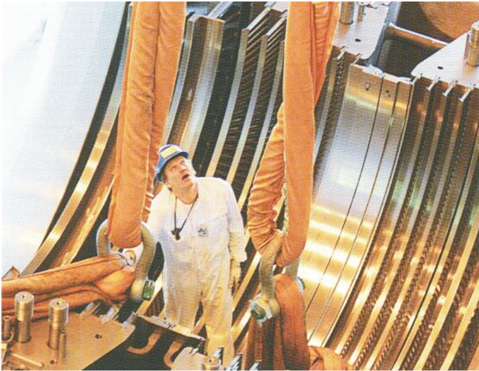
Half of the housing of the low pressure steam turbine stage:
