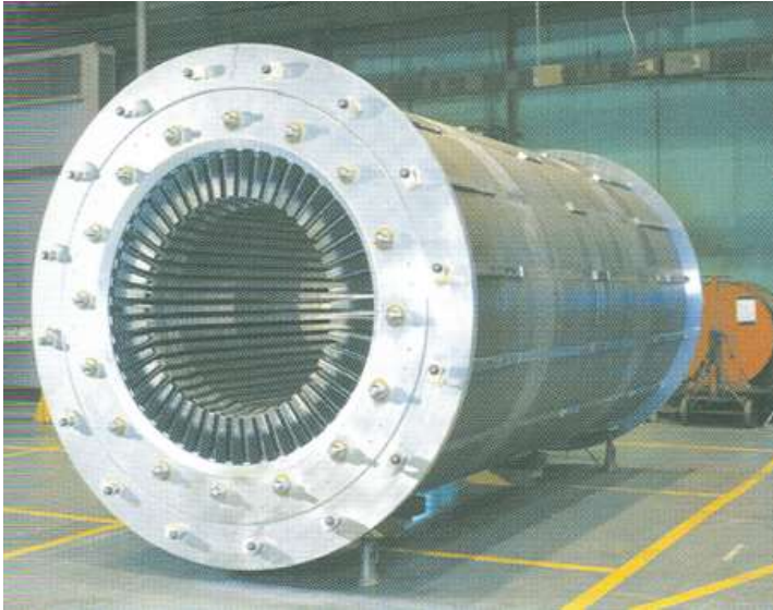
Stator core assembly with bonded stator core packs
