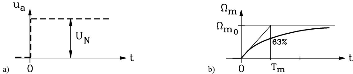
Fig. 5.2.1-2: Dynamic speed response of separately excited DC machine to switching with a) armature voltage step, leading to b) exponential increase of speed
