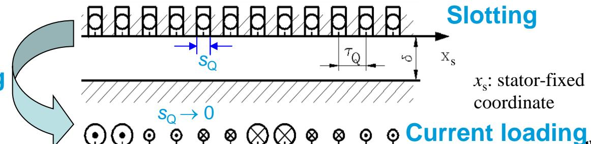
Slotting replaced by “discrete” current loading
