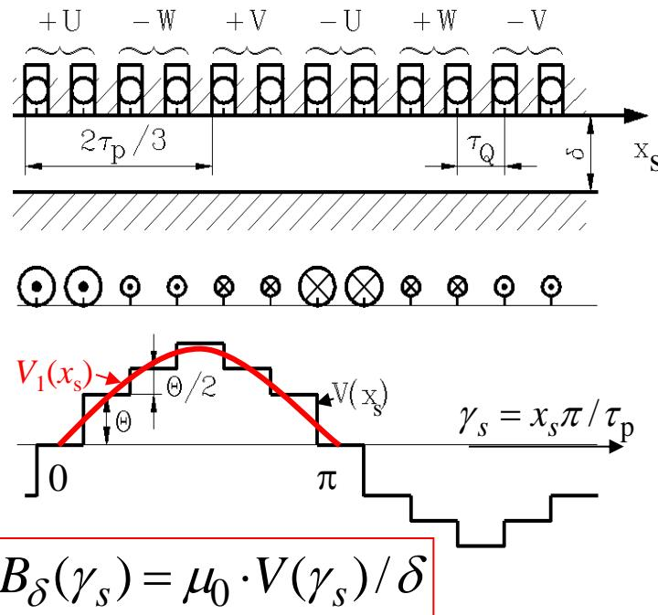
Fundamental of m.m.f. distribution  $V(x_s)$  is a sine wave:
