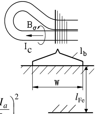
Current density per conductor:  $J = I_c / A_c$       ( $I_c = I_s / a_a$ )
