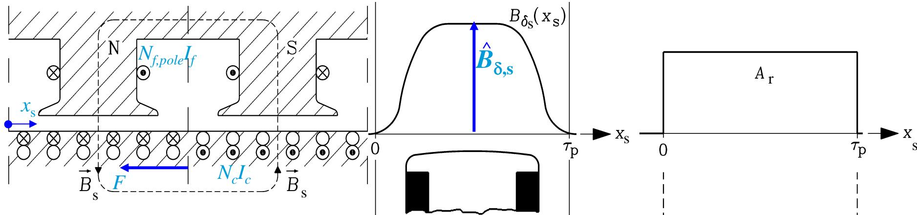
$$\Phi = l_e \int_0^{\tau_p} B_{\delta,s}(x_s) \cdot dx_s = \alpha_e \cdot l_e \cdot \tau_p \cdot \hat{B}_{\delta,s} \quad A_r(x_s) = A_r = \frac{z \cdot I_c}{d_{si} \cdot \pi} = \text{const.}$$
