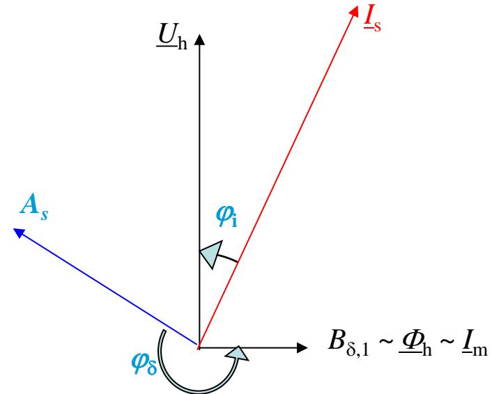
Internal phase angle between internal voltage and stator current:  $\varphi_i = \varphi_\delta - \pi$
