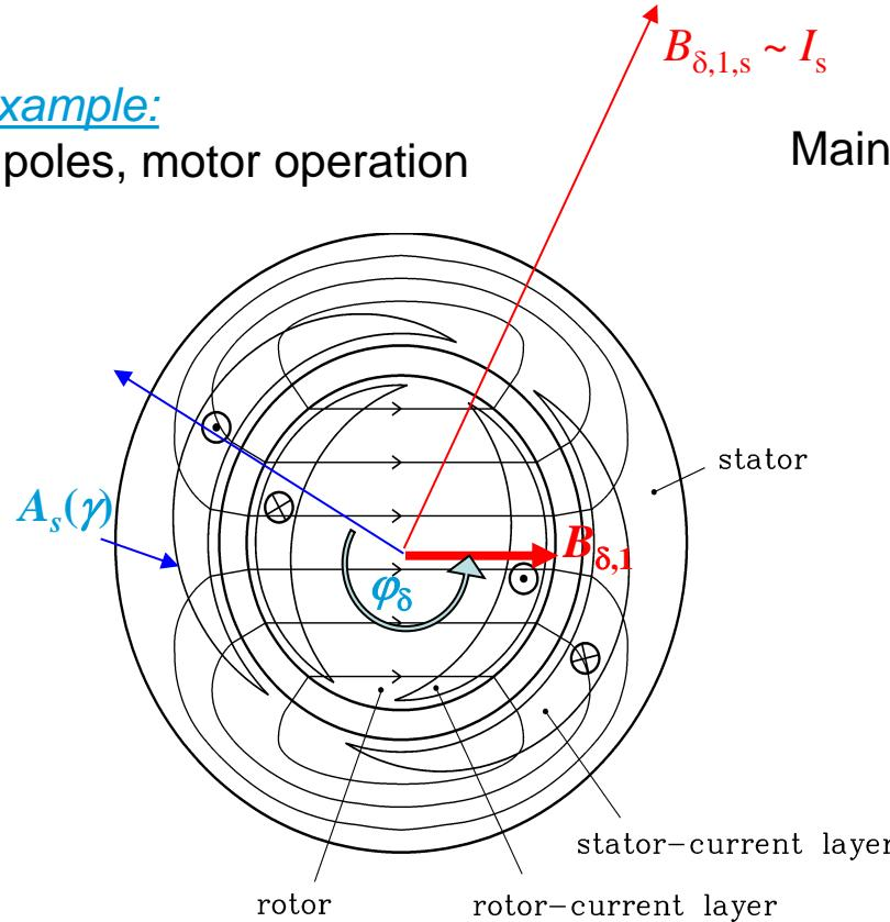
Main flux  $\Phi_h \sim B_{\delta,1} \sim I_m$  and internal voltage  $U_h \sim j \Phi_h$ :
