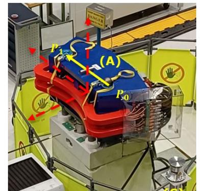
**Figure 1:** Normal conducting H-Magnet.
