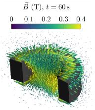
**Figure 1:** Magnetic field of a NI coil computed with 3D FE.
